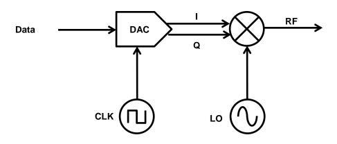
Figure 2. Structure of wireless transmitter using direct conversion
