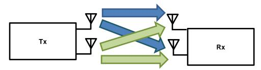
Figure 1. 2x2 MIMO conceptual diagram
