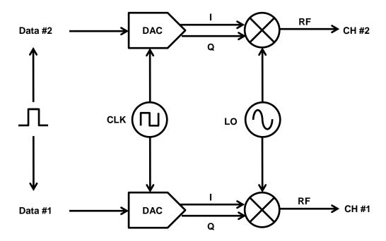
Figure 3. Synchronization between channels
