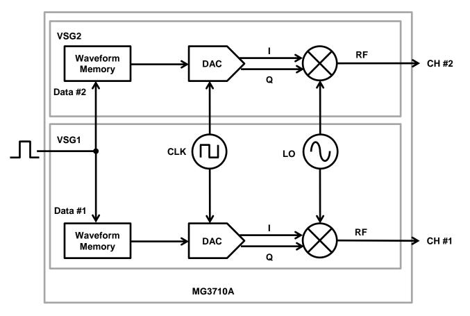
Figure 4. Channel synchronization using MG3710A SG
