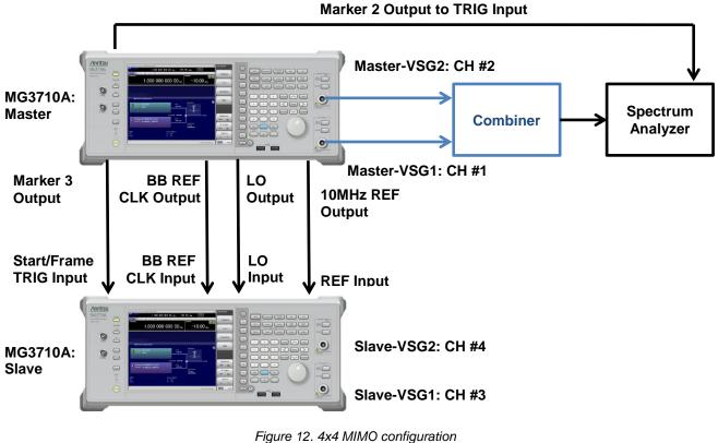
Figure 12. 4x4 MIMO configuration (Connection between Combiner and Spectrum Analyzer is for adjustment to VSG1 and VSG2 in master MG3710A)
