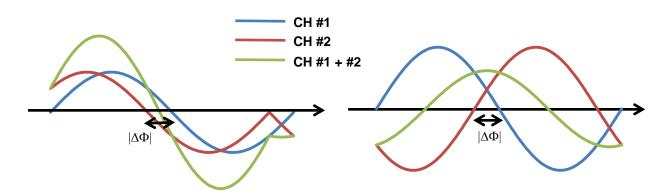
Figure 5. Waveforms of two signals to be synchronized; phase error  $|\Delta \Phi|$  (left) and phase error 180°+  $|\Delta \Phi|$  (right)
